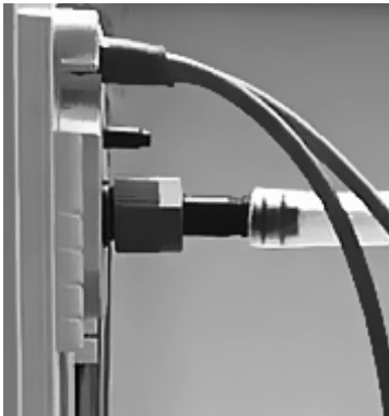
Example 1: vacuum hose made of caoutchouc, directly plugged on the hose nozzle:
